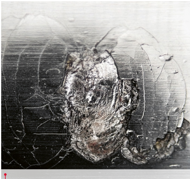
Close up of a material fatigue damage
