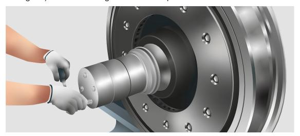
**Step 6:** During cooling, brace the rings with a dummy end cap. Tighten it with the nominal tightening torque (pre-tightening and final tightening torque) of the final end cap.
