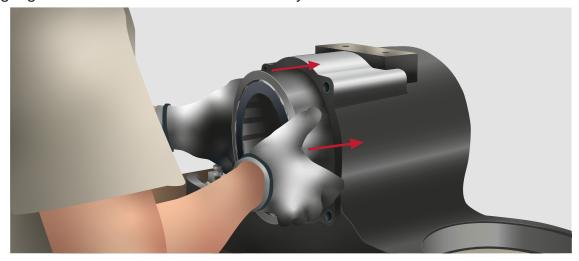
**Step 8:** The two bearing outer rings are pressed into the housing without using force. Light plastic hammer blows on the outer ring are permissible. The housing must not be heated in the process.
