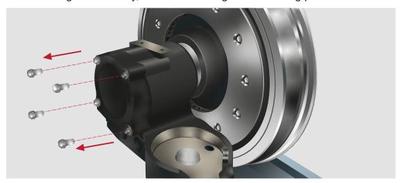
Step 1: Remove the housing cap.
