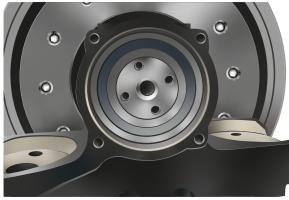
Step 11 (for types WJ+WJP & WJ+WU+HJ): For easier assembly of the loose lip or the L-section ring, heating to approx. 60°C is recommended. Make sure that the markings remain visible during assembly.
