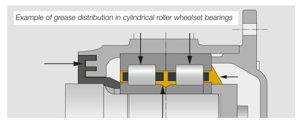
**Step 9:** Ungreased bearings must be filled with grease before the housing is pushed onto the shaft. Make sure that the grease is distributed according to the illustration. The arrows indicate the positions for greasing.
