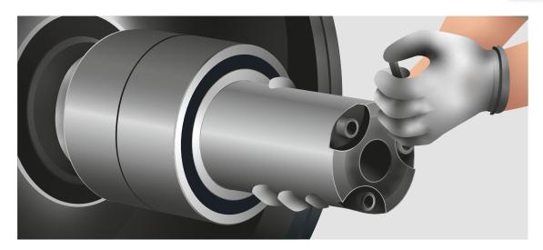
**Step 5:** Before the hydraulic disassembly of the bearing, the mounting sleeve is screwed to the shaft.
