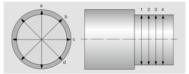
5) The diameter of the cylindrical housing seat is checked with an inside micrometer in four positions in four planes. The following figure shows the measuring points.
