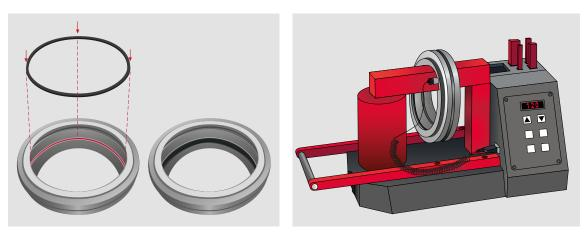
Step 2: Before the assembly of the wheel set bearings, the labyrinth ring is pulled onto the shaft. If an O-ring is available, it must be inserted into the labyrinth ring. The labyrinth ring is inductively heated to approx. 120°C and then pushed onto the shaft. There, it is brought into the correct position with the aid of a stop sleeve. The ring is then allowed to cool for approx. 10 minutes.
