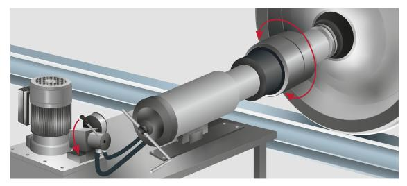
**Step 6:** During the pressing process, the outer ring must be turned by hand to prevent scrape marks on the inner rings.
