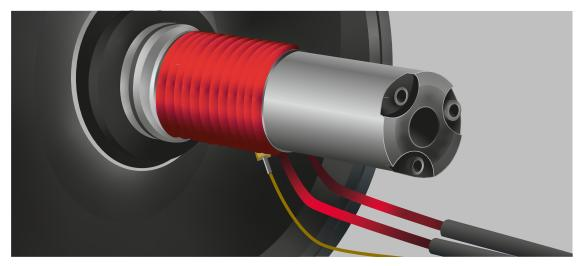
Heating the inner rings by means of an open flame is not permitted.
