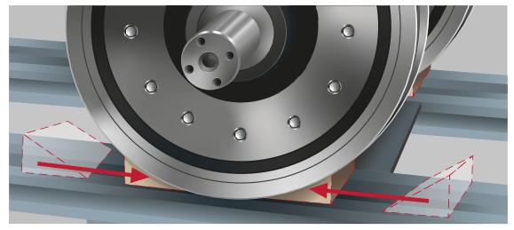
Step 1: Wheel sets shall be locked in place prior to bearing installation.
