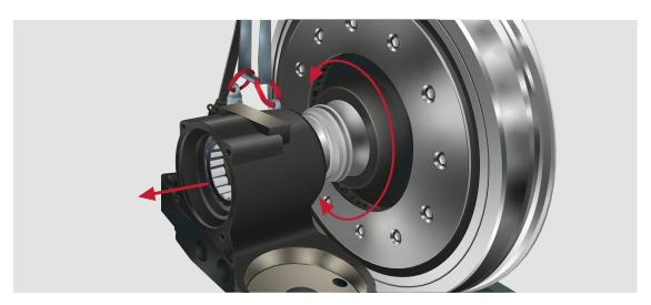
**Step 4:** The housing is pulled from the bearing using an appropriate lifting device. The housing, including the outer ring and the roller and cage assembly, is pulled off the shaft using appropriate lifting equipment. To avoid scrape marks, turn the housing to the left and right by hand during this process.
