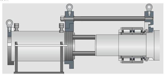
Step 7: Position the extraction tool behind the labyrinth ring.
