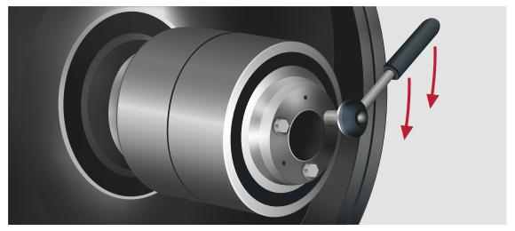
**Step 8:** The pressure cap is fitted and screwed on. The maximum tightening torque can be found in the manufacturer's instructions. Secure the pressure cap according to the manufacturer's specifications.
