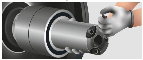
**Step 7:** After the bearing has been pushed completely onto the shaft, the mounting sleeve can be removed.
