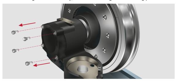
Step 1: Remove the housing cap.
