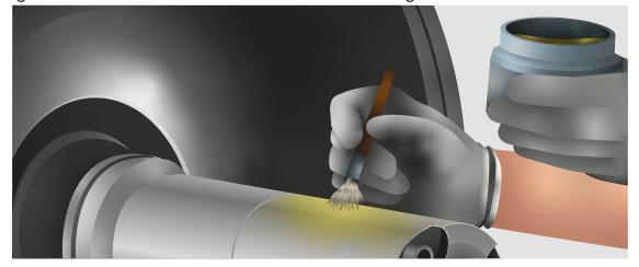
**Step 3:** Apply a thin film of oil to the wheel set shaft to prevent scoring when mounting the bearing.
