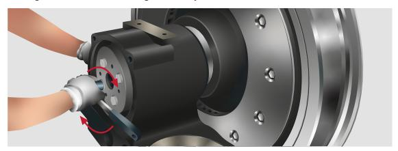
**Step 12:** The pressure cap is fitted and screwed on crosswise. The maximum tightening torque can be found in the manufacturer's instructions. Secure the pressure cap according to these specifications.
