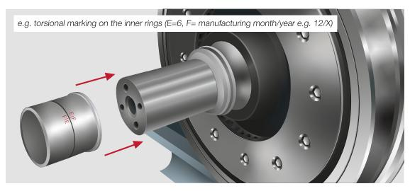
**Step 5:** During the mounting of the inner ring, the line markings on the chamfers or the overrolling-free section of both inner rings must be precisely aligned (torsion marking E/F). The WJ bearing with the fixed lip must be mounted first.
