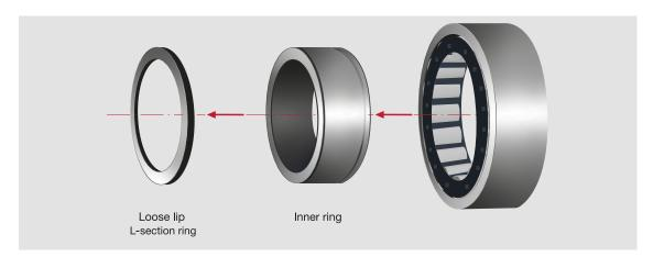
**Step 3:** The inner rings are removed from the bearings by turning them slightly. If there is a loose lip or an L-section ring on one side of the bearings, these must be re-moved beforehand and repositioned in the same place during the installation of the outer ring / roller and cage assembly. In the case of sealed rolling bearings, ensure that the seals are not damaged and that only small quantities of grease escape from the bearing during inner ring removal.
