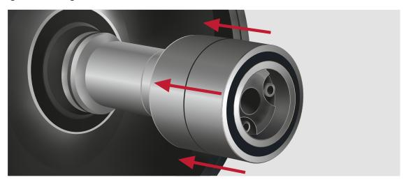
**Step 4:** Slide the wheel set bearing unit, labyrinth ring first, to the end of the mounting sleeve without canting. Slight turning can prevent the formation of scrape marks. For sealed rolling bearings, make sure the sealing ring does not slip out of the seal cap.
