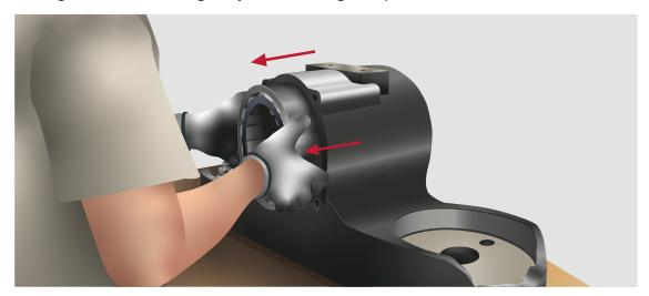
**Step 5:** Push the outer rings with the roller complement out of the housing. If extraction tools are used for this purpose, make sure that they do not damage either the rolling elements or the cage. The disassembly forces must not be transmitted via the rolling elements.
