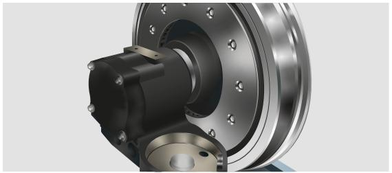
**Step 10:** Finally, check whether the bearing has been mounted correctly. For this purpose, smooth running is checked by axial shifting and rotation. If irregularities occur, the bearing must be disassembled from the shaft and the cause determined.
