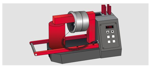
**Step 4:** The inner rings are heated evenly to a maximum of 120°C using an induction heating device or a heating plate. To prevent an overheating of the bearing parts, the heating temperature must be controlled. Inductively mounted bearing parts must be demagnetized.
