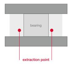
Simplified representation of the extraction points outside of the cage on the bearing end faces
