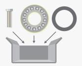
Pack the rolling bearing in a dismounted state. Please do not remove lubricants etc. from the bearing. Make sure that all components, seals and a lubricant sample are packed.
