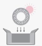
Pack the rolling bearing in a dry and clean condition. Make sure that all components are packed.
