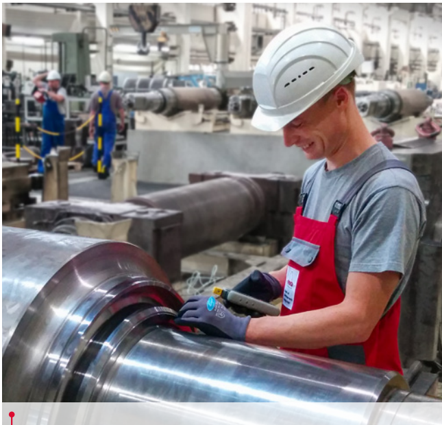
KRW employee checking the inner ring temperature during rolling bearing mounting
